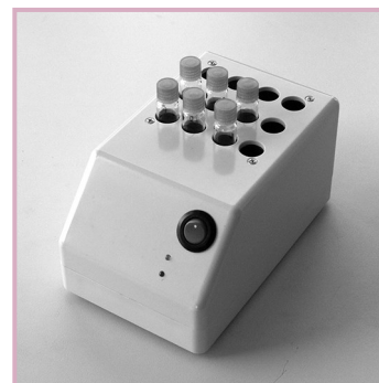
3. Close cuvettes, mix and insert them immediately into the dry block thermostat
